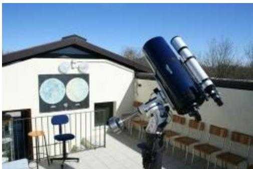
Inside the observatory lie various telescopes. Among these, the main telescope: a 14" Schmidt-Cassegrain Meade which, along with its accessories, is controlled by an internal command station. In addition, the observatory can vaunt a CCD Sbig ST10, a solar filter, and many other state of the art technologies.
